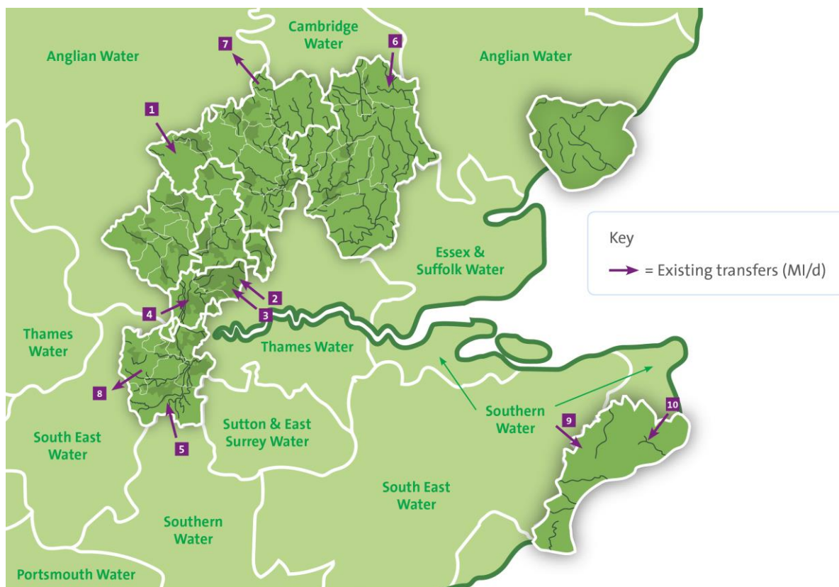
Figure 22: Location of existing import and export arrangements (numbers relate to transfer IDs)
